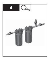
Remove both the housings using sump wrench.
