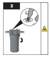
Press the pressure button to release the pressure from the cartridges
